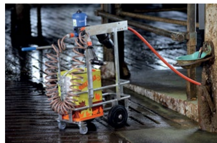
"With the dosing device we apply GÜLLEMAX as a 5% solution on walls and floors."
